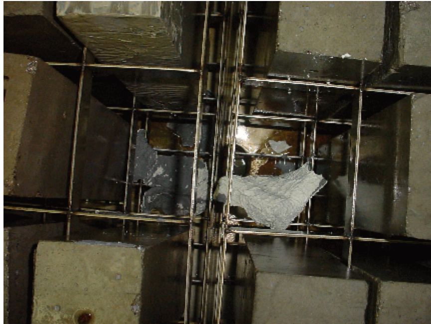
PORTIONS OF THE COATING THAT CAME OFF DURING THE TEST
