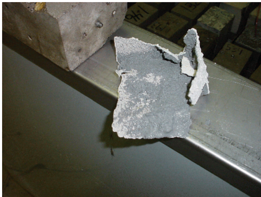
PORTIONS OF THE COATING THAT CAME OFF DURING THE TEST
